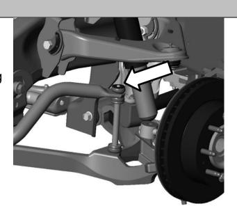
Repeat the above steps for removing the sway bar end link on the opposite side of the vehicle.
