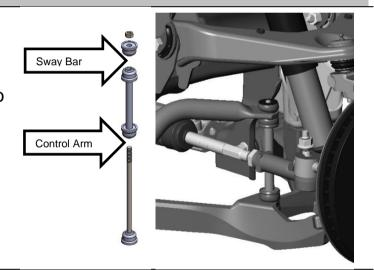
Repeat the above steps for installing the other sway bar end link on the opposite side of the vehicle.
